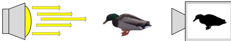
Fig. 2.4 Backlighting. The light source is behind the object of interest, which makes the object stand out as a black silhouette. Note that the details inside the object are lost
